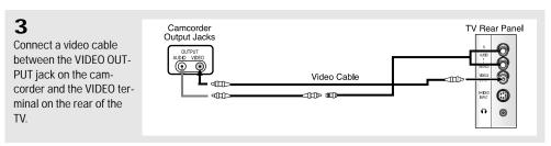
The audio-video cables shown here are usually included with a Camcorder. (If not, check your local electronics store.) If your camcorder is stereo, you need to connect a set of two cables.
